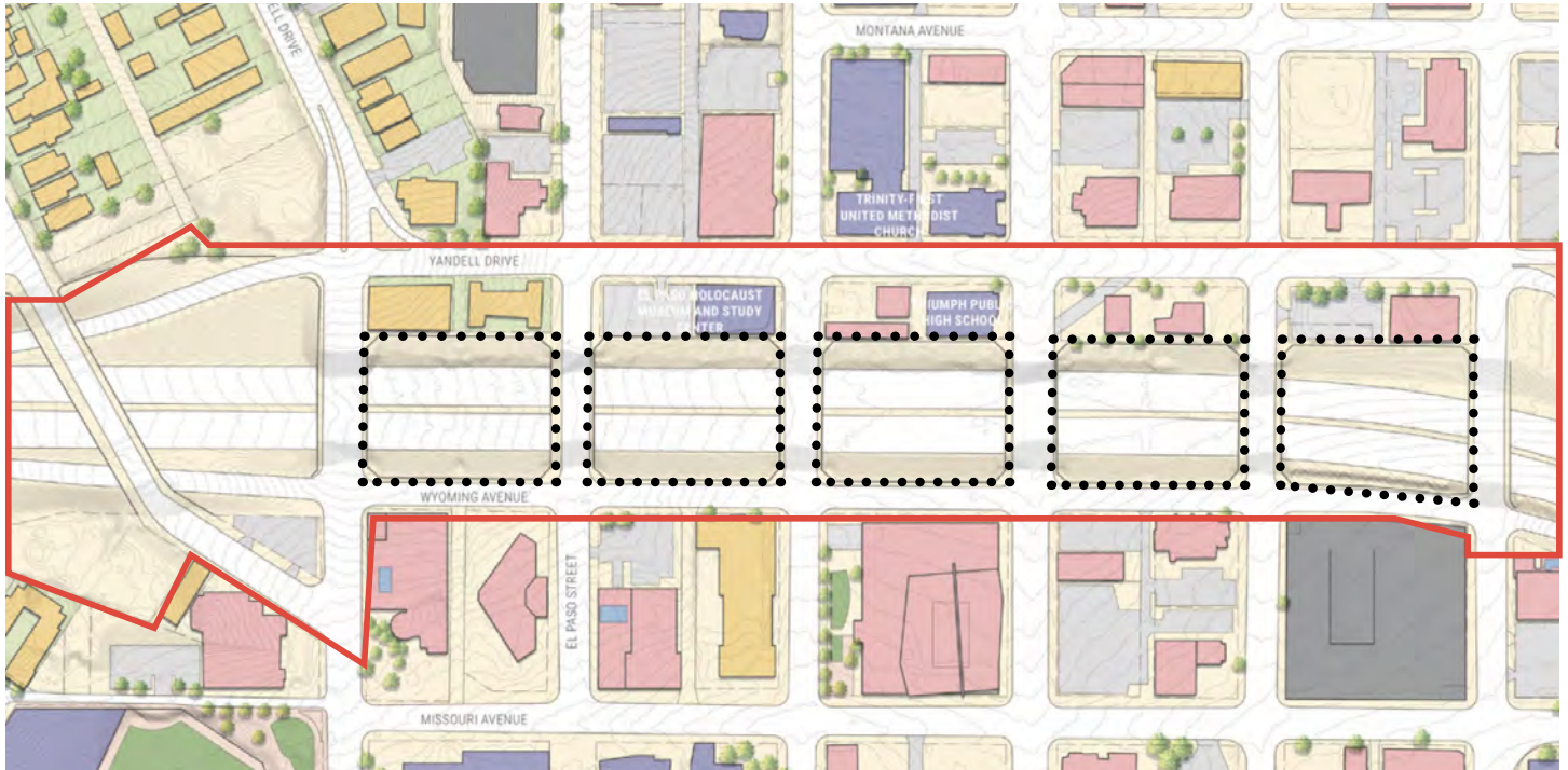
Plan of existing conditions showing the proposed decked areas and the right-of-way for the I-10 study.
